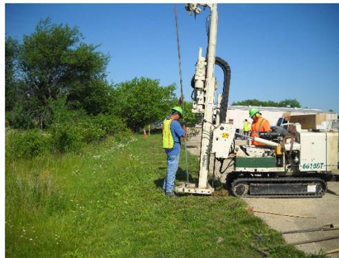
Figure 3: Direct Push Technology Drill Rig
